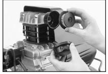
Figure 15. Air filter element.
